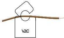
2. Locate the phase supplying the whole installation and connect the clamp meter. Release the sensor and fit around the power cable. Close the clip to hold it firmly in place. Normally, this is the connection from the meter, which is grey, black or brown. If it is a three-phase installation, you must use the 3 clamps (view slave graphic) and must all previously exposed cables. **IMPORTANT:** the clip should cover the ENTIRE phase to read the energy of the whole installation (house + e-Charger).
