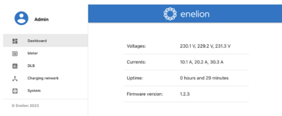
Fig. 8: View of the Dashboard section in the EEG 3.0 configuration panel
